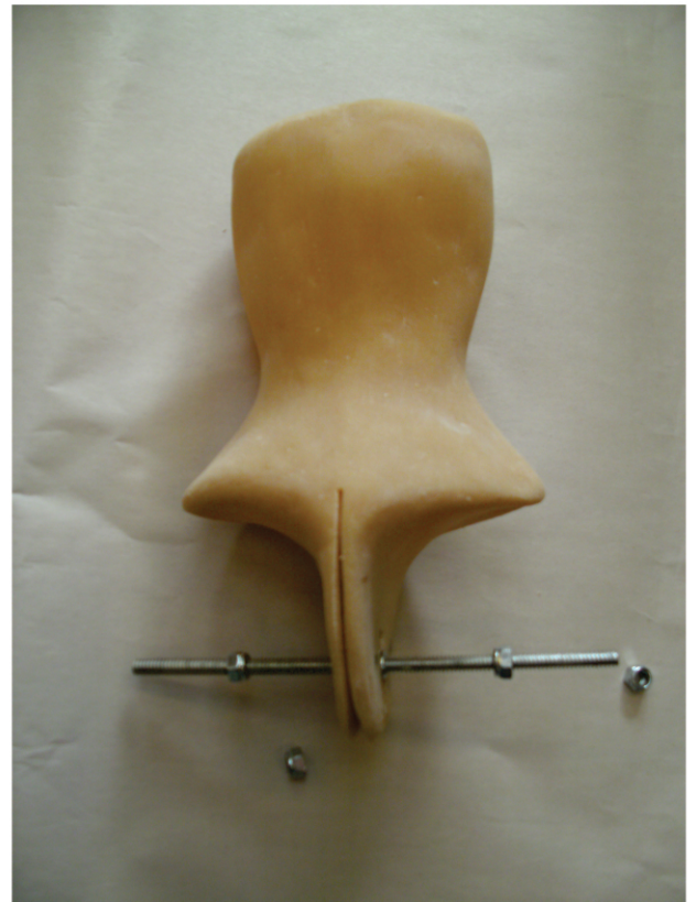
The crutch set up with a threaded rod and lock nuts to take the upper leg.
